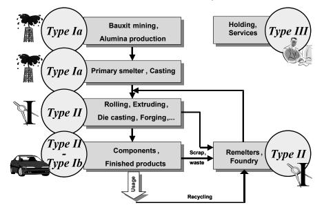
Fig. 13. The value-add chain of the aluminium industry
