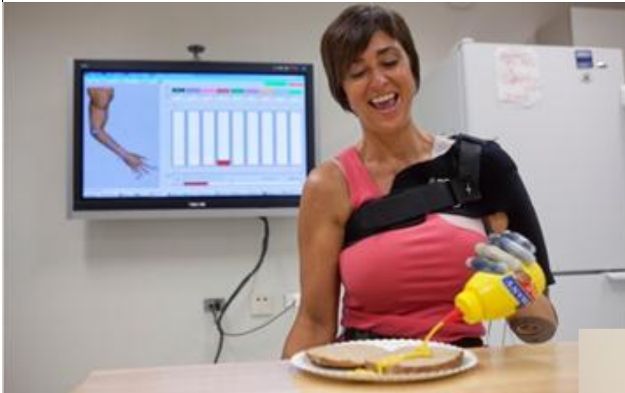
Fig. 6. Amanda Kitts using her bionic arm to squirt mustard
